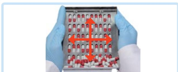
2 Pour some capsules onto feeder. Shake slightly until capsules cover all slots.
