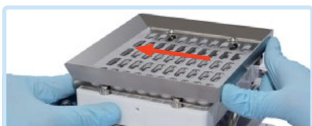
4 Place feeder locating feet in front holes of Caps Tray. Slide Orienter Tray to the left till all capsules drop. Repeat the same action by placing feeder locating feet in second holes (II).
