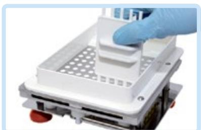
**11a** Tapping: Pull cam lever to gently hold capsule bodies in place. Hold Filler Base frame and tap against table a few times to settle powder.
