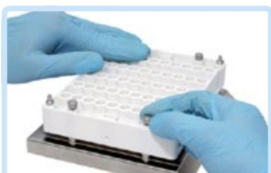
5 Attach Orienter Base to Orienter Tray with four screws.
