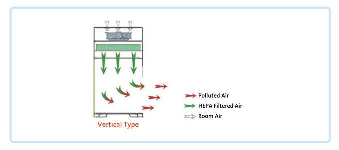
Laminar flow cabinet LF-800 UV creates a local high cleanliness air environment by vertical air flow. It is widely used in preparation process of compounded medication in compounding pharmacies specially when contamination risk is high in the working environment. It is suggested to be used in high or medium risk preparations.
