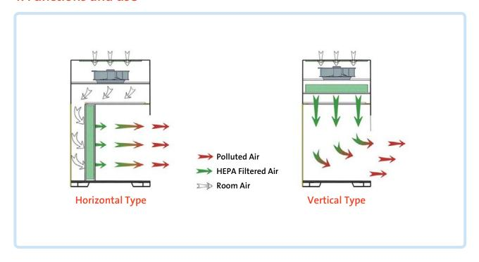
Laminar flow cabinet LF-800 UV creates a local high cleanliness air environment by vertical air flow. It is widely used in preparation process of compounded medication in pharmacies specially when contamination risk is high in the working environment. It is suggested to be used in high or medium risk preparations.
