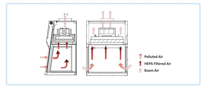
Laminar flow cabinet NP-800 UV creates a local high cleanliness air environment by vertical air flow. It is widely used in preparation process of compounded medication in compounding pharmacies to protect user from inhaling dangerous substances. It is recommended during mixing and capsule filling of such substances. It is very helpful to increase yield, precision, stability and reliability of products.
