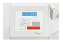
1. Press the "STOP" button to pause the mixing cycle.
