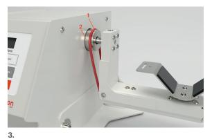
To fit the inversion arm, place the orange belt (1) over the pulley (2).
