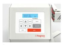
**3.** When the time has elapsed, the mixer will stop and a buzzer will sound.
