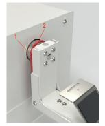
**4.** Keep tension on the orange belt (**1**) and push the arm downwards onto the driveshaft (**2**).
