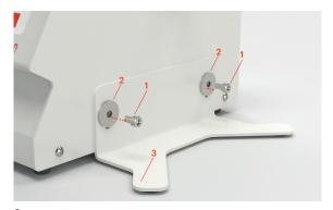
2. Fit the stabilizer (3), push it down (3), and fit washers (2) and screws (1).
