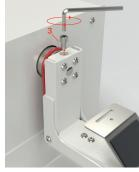
**5.** Tighten the screw with the tool supplied. Ensure the screw (**3**) is on the flat portion of the driveshaft.
