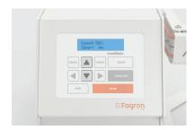
3. Adjust the timer by using the "UP" ▲ and "DOWN" ▼ buttons.
