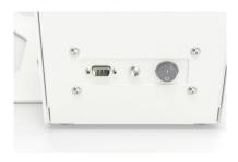
1. InvoMatic is equipped with a Serial RS232 port, suitable for different models of thermal printers.
