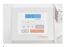
1. After setting the desired speed and time, press the "RUN" button. The mixer will begin to rotate.
